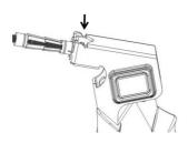
Place the hollow nail into the perforated member and press the handle to inflate the hollow nail into shape until it is firmly on th member.
